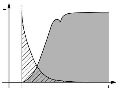
Compared with solenoid valves, proportional valves with piezo technology require virtually no energy to maintain an active state, thanks to their capacitive principle. The piezo valve operates like a capacitor: it needs current only at the start in order to charge the piezoceramics.
